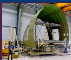
Sub-assembly of Section 11/12, Méaulte
